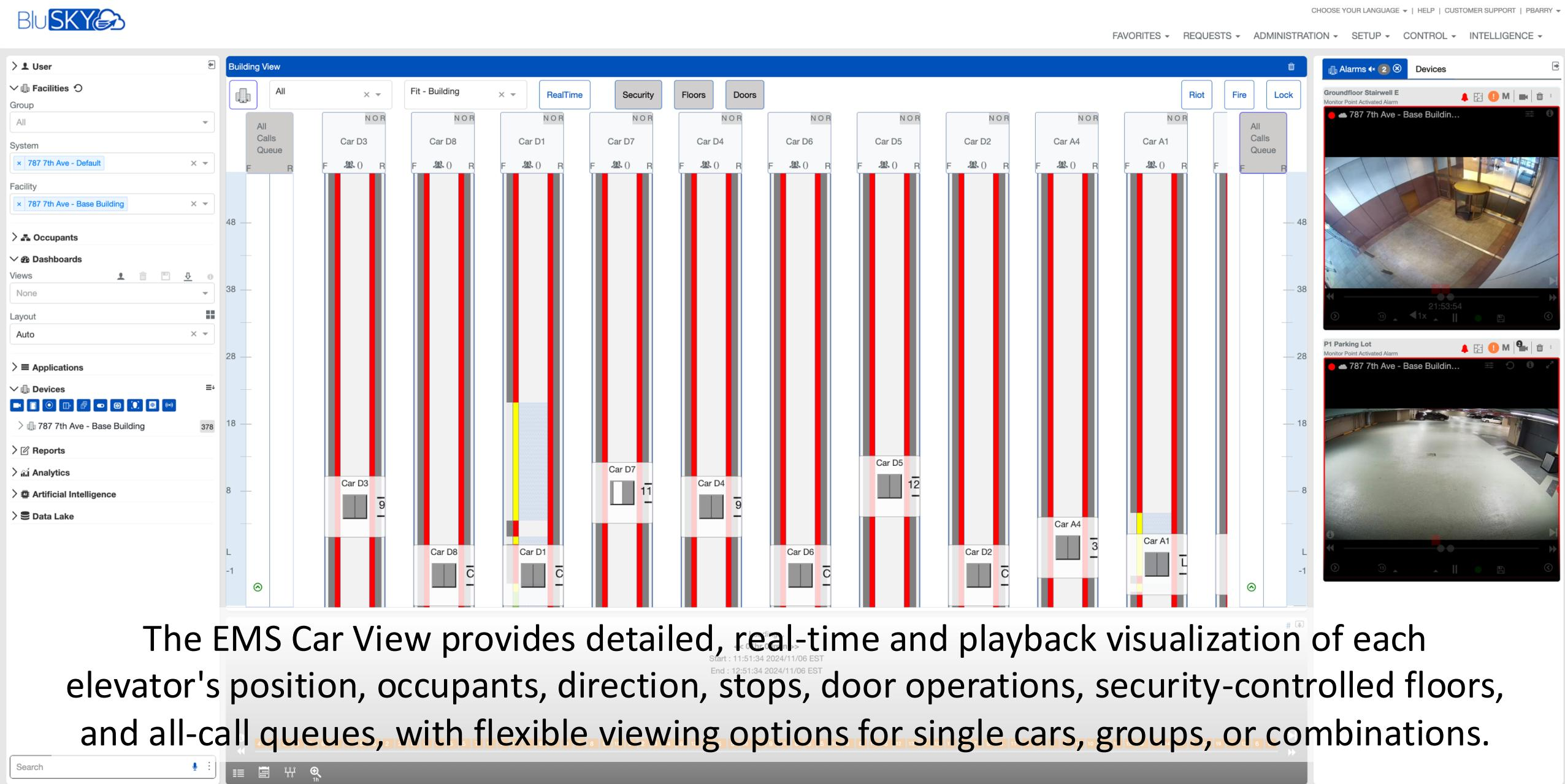
The EMS Car View provides detailed, real-time and playback visualization of each elevator's position, occupants, direction, stops, door operations, security-controlled floors, and all-call queues, with flexible viewing options for single cars, groups, or combinations.
