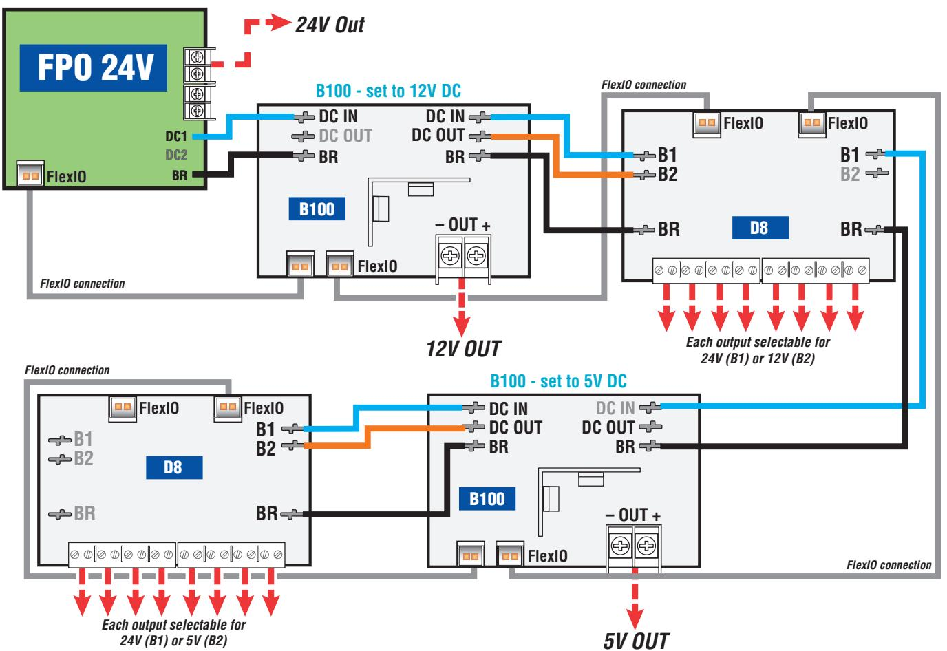
**B100 Application Examples****Triple Voltage (24V/12V/5V) using two FPO's, one B100 with 8 output distribution**
