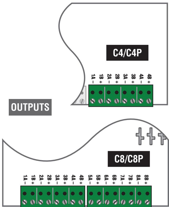
Each input on the **C4** and **C8** has an “A” terminal and a “B” terminal.
