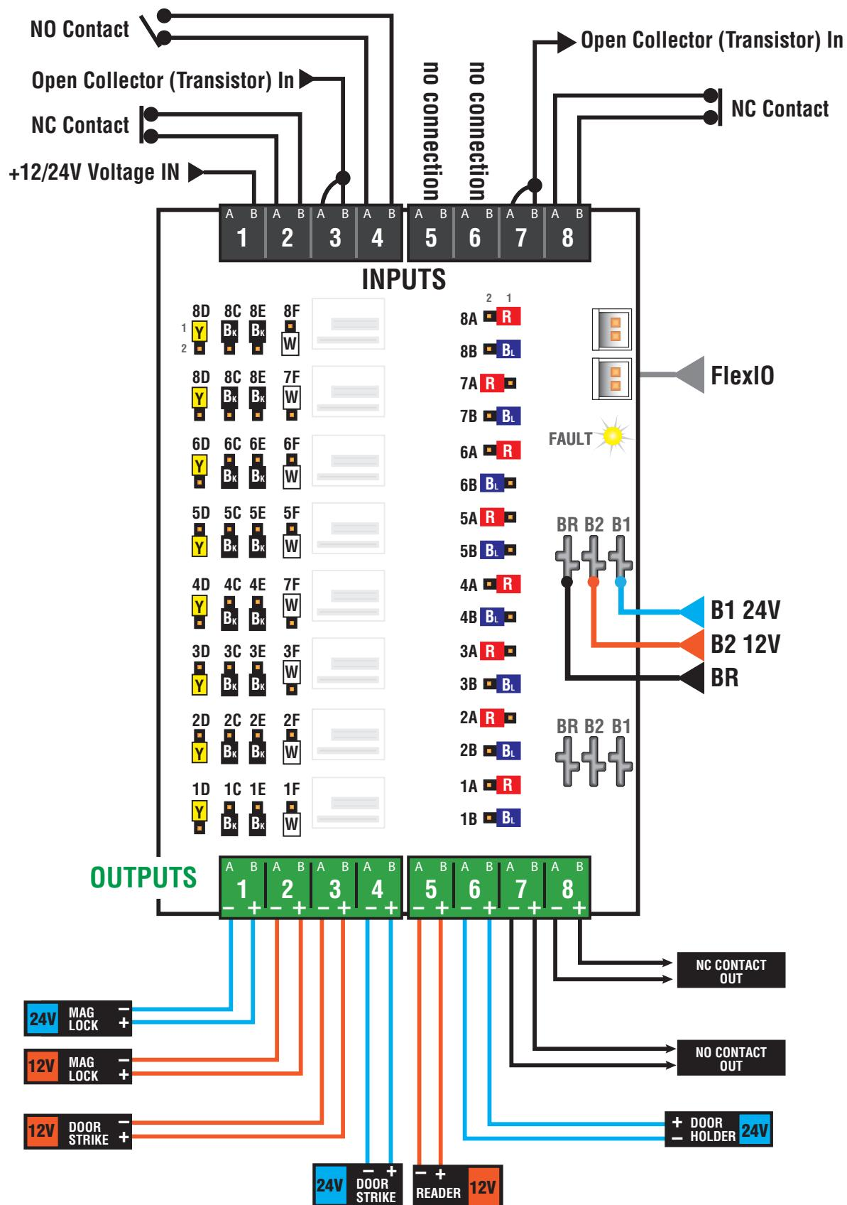
**Zone 1****24V Mag Lock Output, Voltage Input, with FAI**
