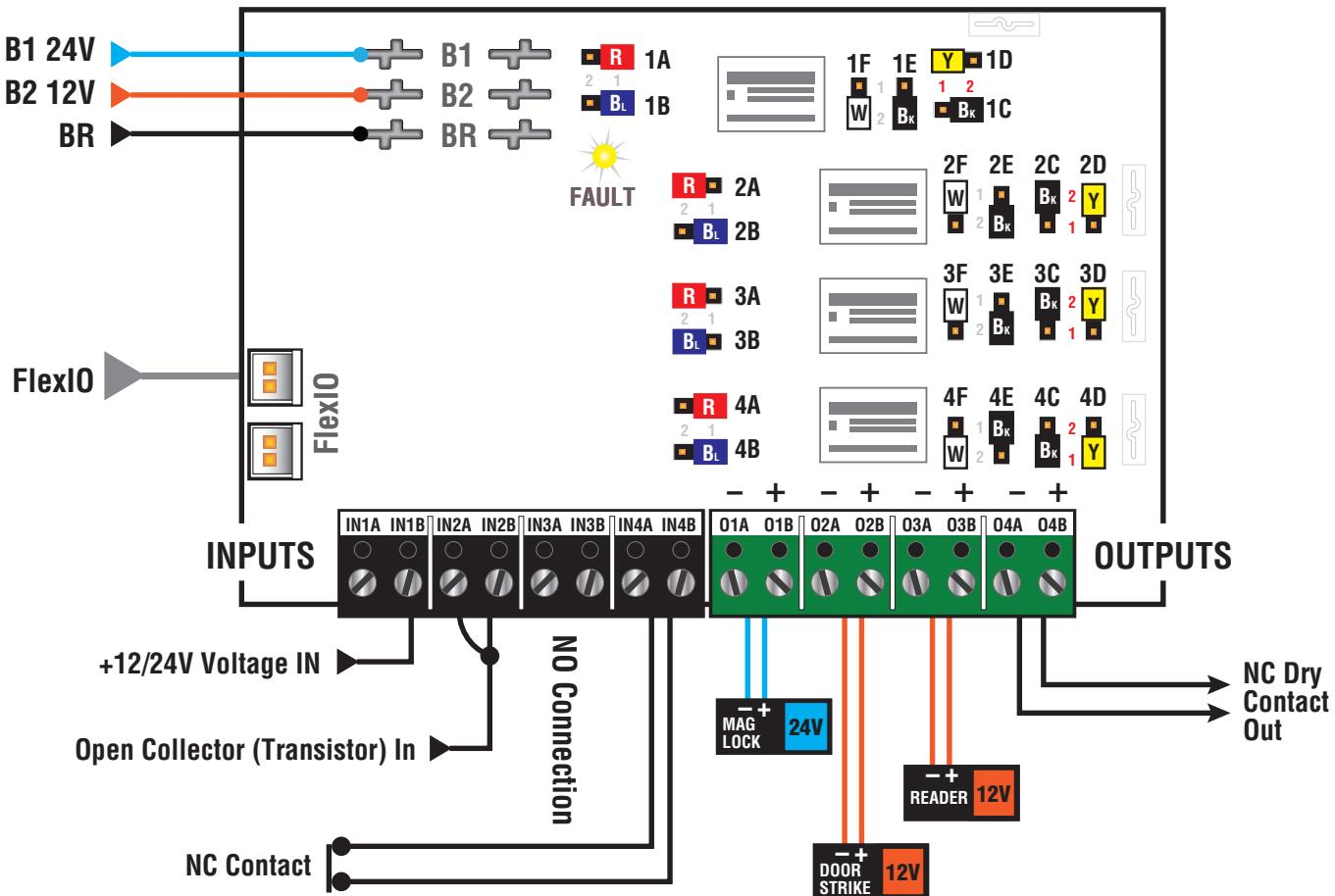
**Zone 1****24V Mag Lock Output, Voltage Input, with FAI**
