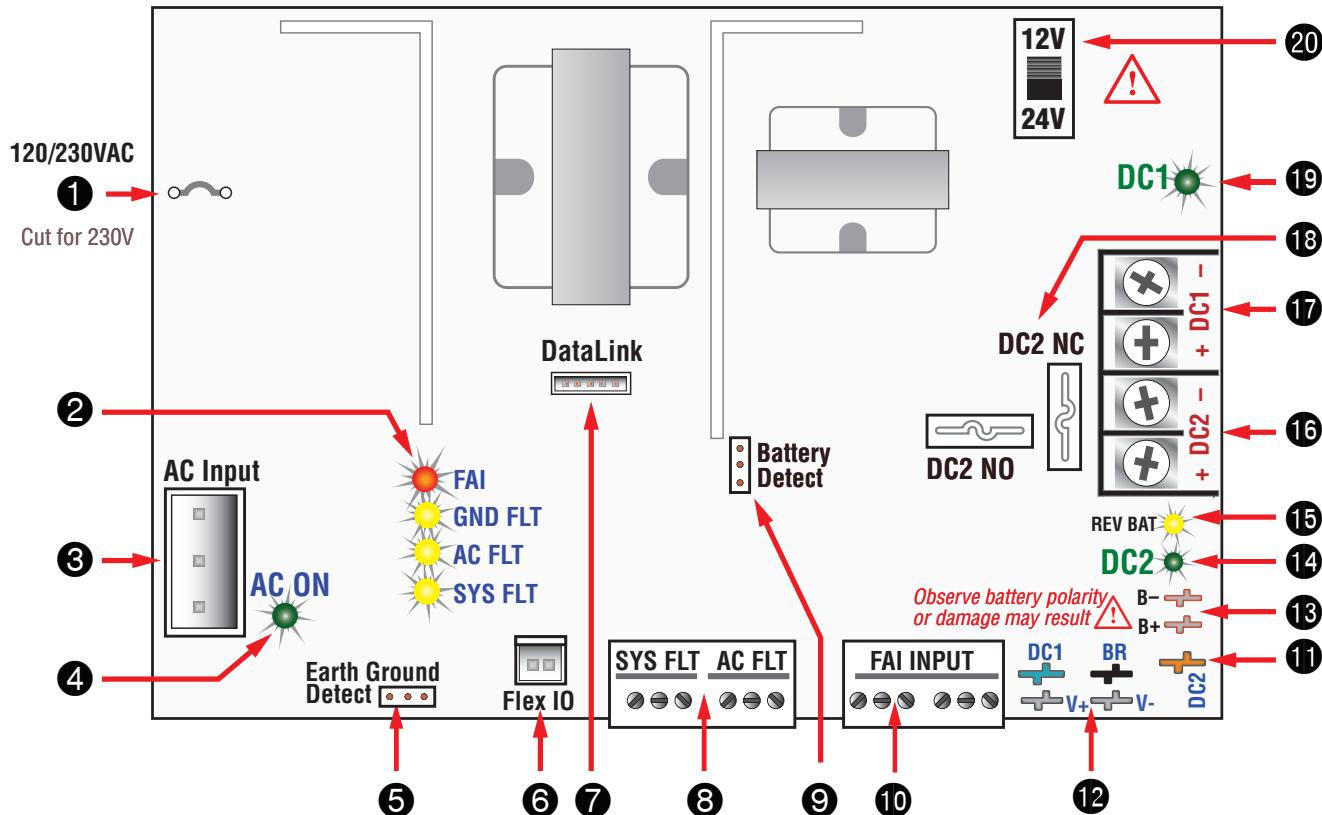
**9** **Battery Presence Detection (JP3)** The BAT DET jumper enables or disables Battery Presence (BP) fault detection as follows:
