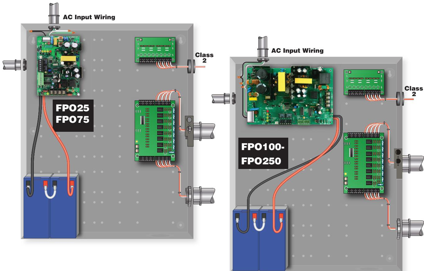
The drawing above shows a typical installation.
